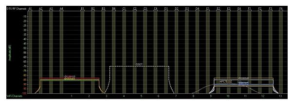
It can be readily seen that in the above circumstances, MDTS radio channels A1, D2, D3 and F4 are open or not being used by other radios identified in the immediate vicinity.
