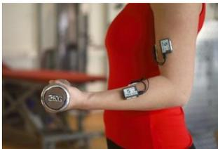
The EMG Sensors can be secured in place using Noraxon supplied double-sided adhesive tape and/or elastic straps. Straps are recommended if dynamic movements are expected.
