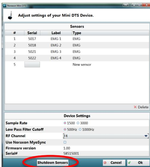
When the sensors are shutdown they will stop blinking completely. The sensors are reactivated by briefly charging them.
