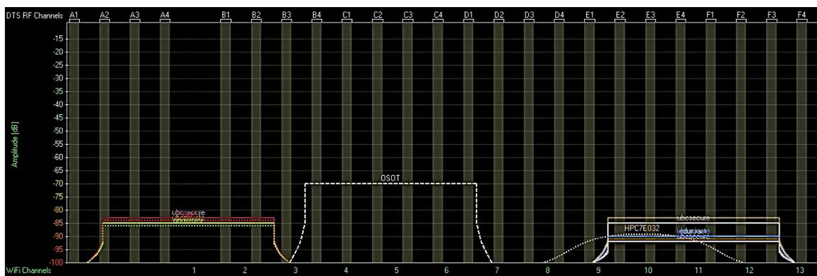
It can be readily seen that in the above circumstances, MDTs radio channels A1, D2, D3 and F4 are open or not being used by other radios identified in the immediate vicinity.
